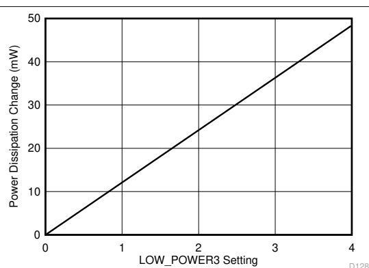
图 9-13. Power Dissipation Change vs LOW_POWER3 register setting
