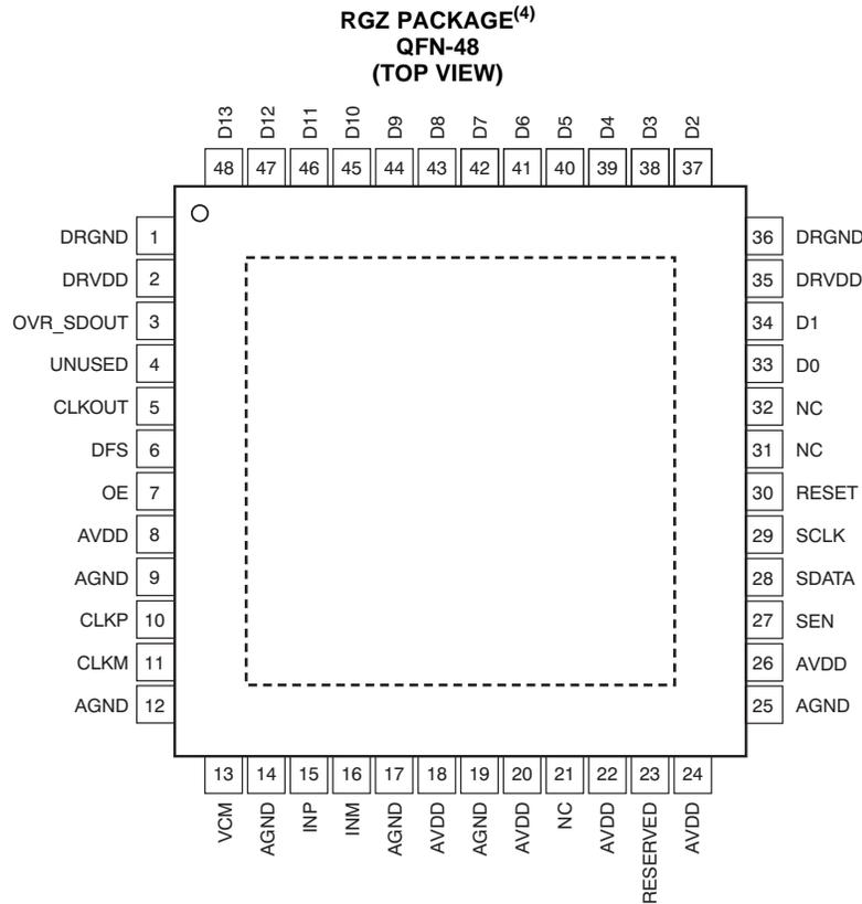
(4) The PowerPAD is connected to DRGND.
