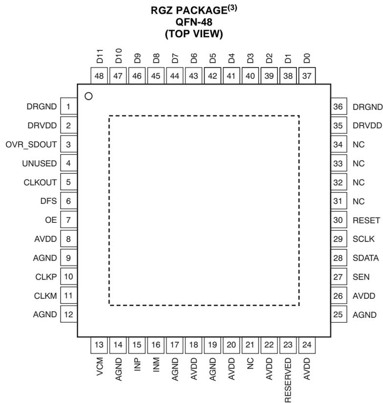
(3) The PowerPAD is connected to DRGND.
