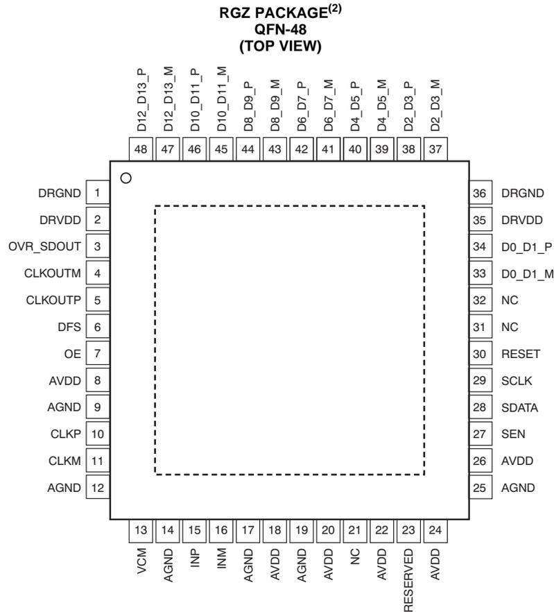
(2) The PowerPAD™ is connected to DRGND.
