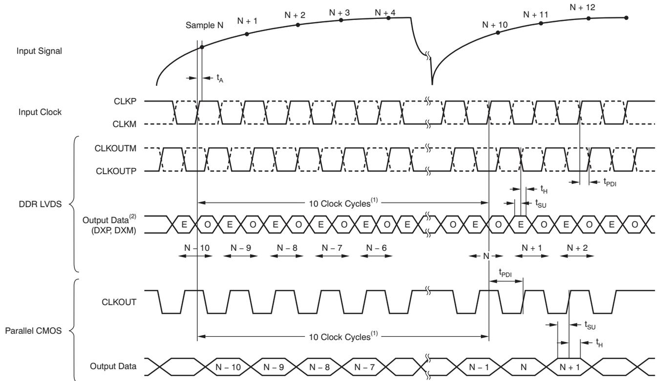
(1) ADC latency in low-latency mode. At higher sampling frequencies,  $t_{PD1}$  is greater than one clock cycle which then makes the overall latency = ADC latency + 1.
