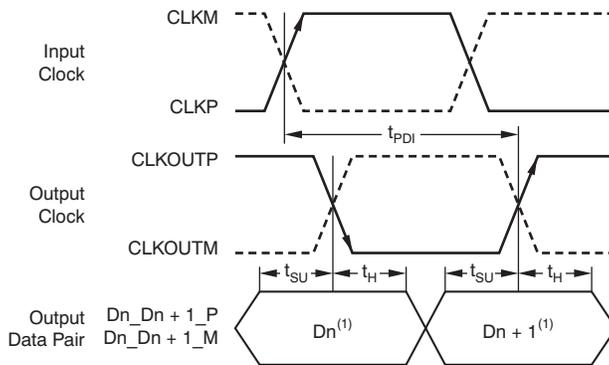
(1)  $D_n$  = bits D0, D2, D4, etc.  $D_{n+1}$  = Bits D1, D3, D5, etc.
