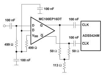
Figure 23. Differential Clock Using PECL Logic
