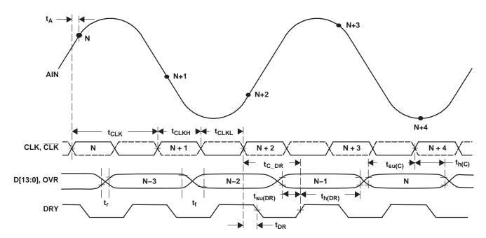
Figure 1. Timing Diagram
