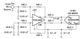
Figure 20. Using the THS4509 With the ADS5424
