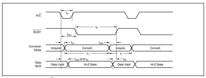
FIGURE 6. Convert Mode: R/C Pulse LOW — Outputs Enabled After Conversion.
