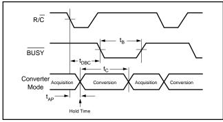
FIGURE 3. Acquisition and Conversion Timing.
