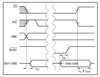
FIGURE 9. Read Cycle Timing.
