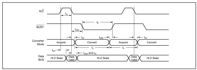
FIGURE 7. Read Mode:  $R/\overline{C}$  Pulse HIGH— Outputs Enabled Only When  $R/\overline{C}$  is High.
