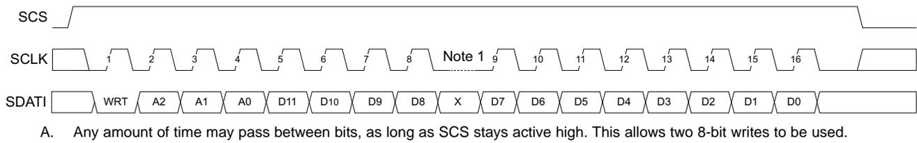
**Figure 17. Write Operation**
