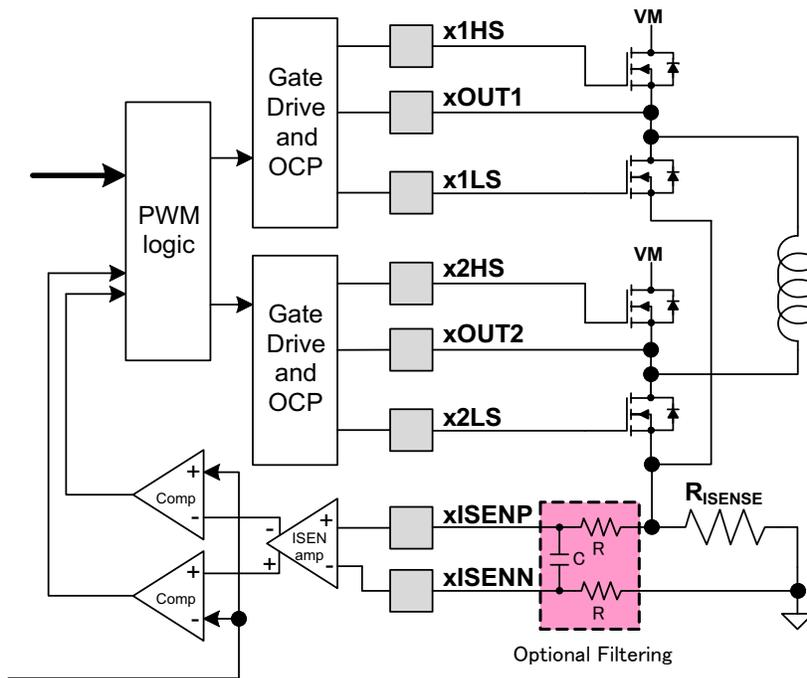
Figure 12. Optional Filtering Between  $R_{ISENSE}$  and xINSENx
