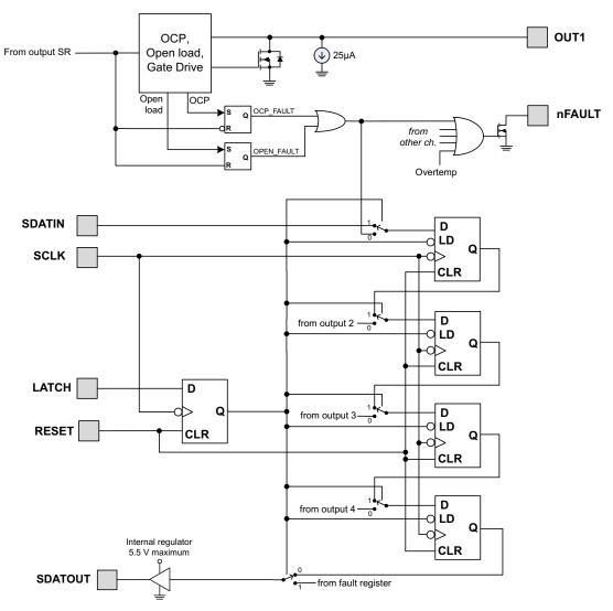
Figure 7. Fault Output
