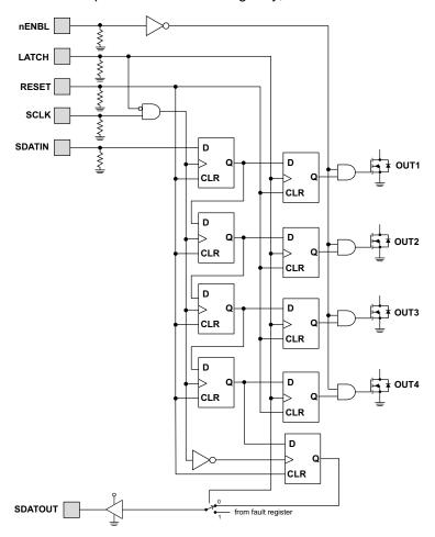
Figure 6. Serial Interface Operation
