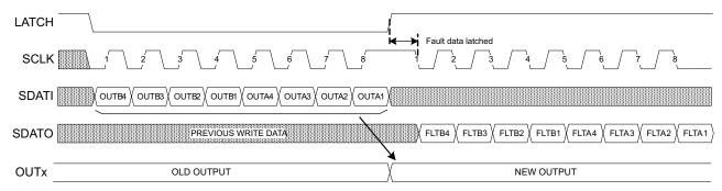
Figure 9. Daisy-Chain Serial Transaction
