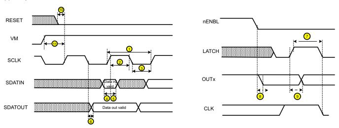
More than 400 ns of delay should exist between the final SCLK rising edge and the LATCH rising edge. This ensures that the last data bit is shifted into the device properly.
