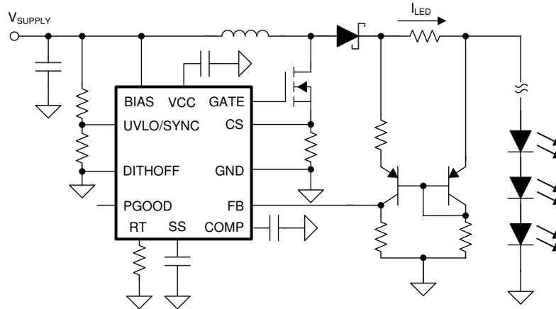
图 10-13. LED Driver with High-Side Current Sensing
