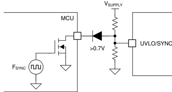
图 9-14. UVLO, Standby, and Clock Synchronization (a)
