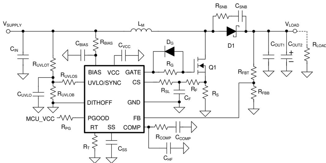
图 10-1. Typical Boost Converter Circuit With Optional Components
