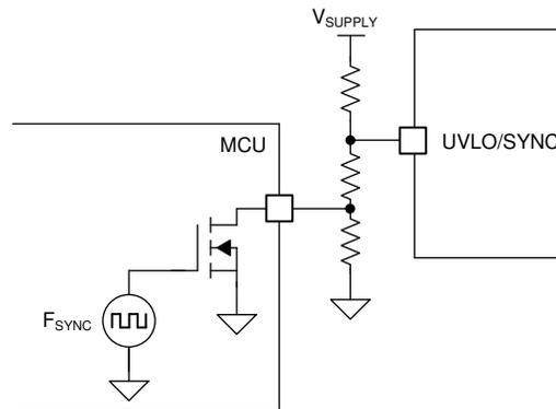
图 9-15. UVLO, Standby, and Clock Synchronization (b)
