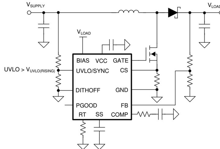
图 9-6. Decrease the Minimum Operating Voltage After Start-Up
