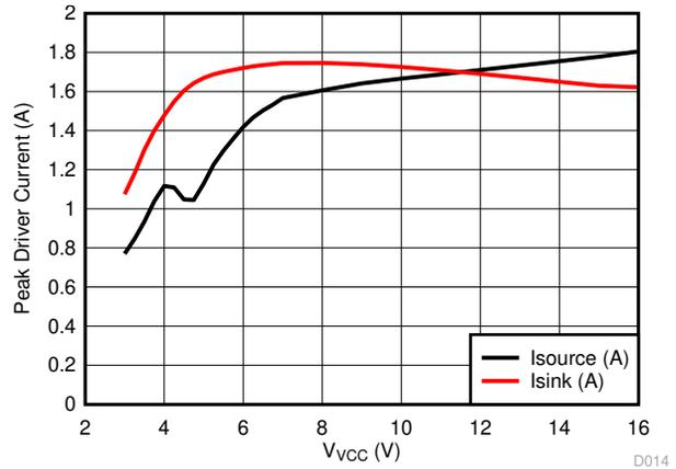
图 8-14. Peak Driver Current vs V<sub>CC</sub>
