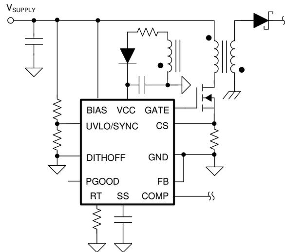
图 9-7. External VCC Supply ( $BIAS \geq VCC$ )
