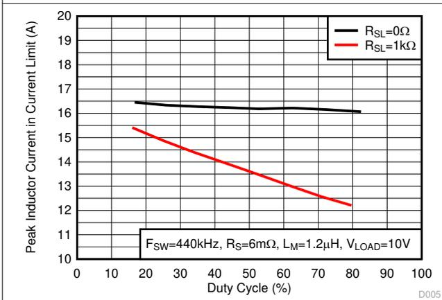
图 8-5. Peak Current Limit vs Duty Cycle
