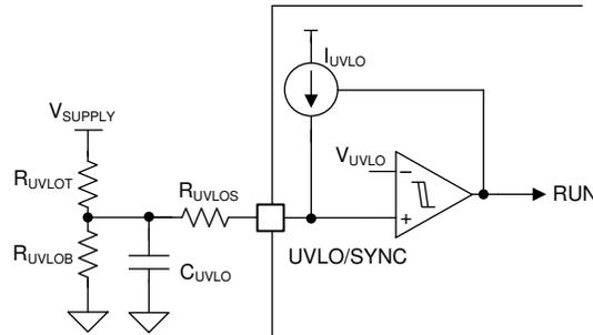
图 9-4. Line UVLO Using Three UVLO Resistors
