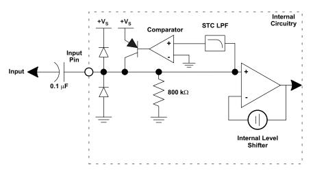
Figure 6. Equivalent AC Sync-Tip Clamp Input Circuit
