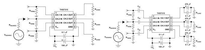
Figure 1. DC-Coupled Input and Output Test Circuit
