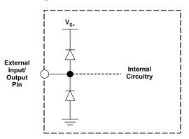
Figure 3. Internal ESD Protection
