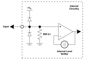
Figure 5. Equivalent DC Input Mode Circuit
