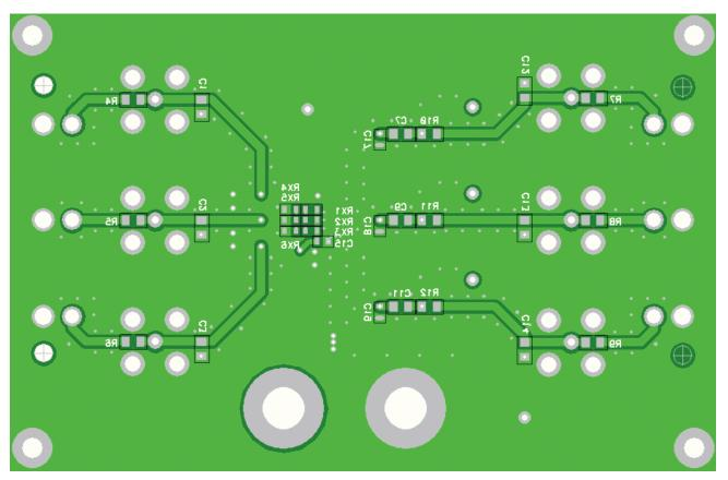
Figure 12. THS7315D EVM PCB Bottom Layer
