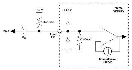
Figure 7. AC-Bias Input Mode Circuit Configuration
