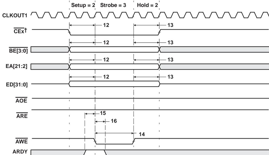
† If no write accesses are scheduled for the next cycle and write hold is set to 1 or greater, then  $\overline{\text{CE}}_{\text{x}}$  stays active for three cycles after the value of the programmed hold period. If write hold is set to 0, then  $\overline{\text{CE}}_{\text{x}}$  stays active for four more cycles. This does not affect performance, it merely reflects the EMIF's overhead.
