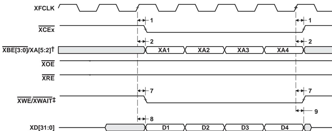
†  $\overline{XBE}[3:0]/XA[5:2]$  operate as address signals  $XA[5:2]$  during synchronous FIFO accesses.
