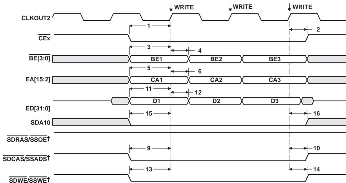
†  $\overline{\text{SDCAS}}/\overline{\text{SSADS}}$ ,  $\overline{\text{SDRAS}}/\overline{\text{SSOE}}$ , and  $\overline{\text{SDWE}}/\overline{\text{SSWE}}$  operate as  $\overline{\text{SDCAS}}$ ,  $\overline{\text{SDRAS}}$ , and  $\overline{\text{SDWE}}$ , respectively, during SDRAM accesses.
