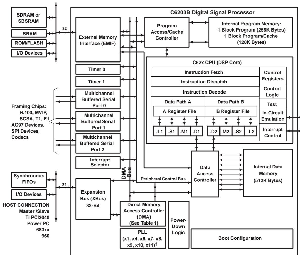
† For additional details on the PLL clock module and specific options for the C6203B device, see Table 1 and the *Clock PLL* section of this data sheet.
