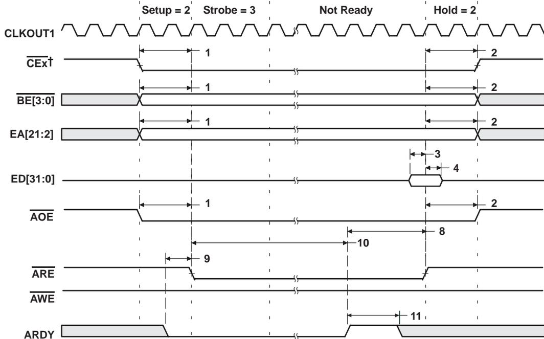
†  $\overline{\text{CE}}$  stays active for seven minus the value of Read Hold cycles after the last access (DMA transfer or CPU access). For example, if read HOLD = 1, then  $\overline{\text{CE}}$  stays active for six more cycles. This does not affect performance, it merely reflects the EMIF's overhead.
