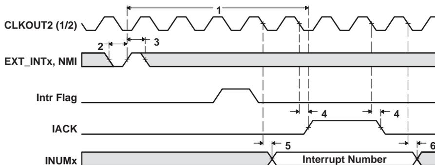
Figure 33. Interrupt Timing
