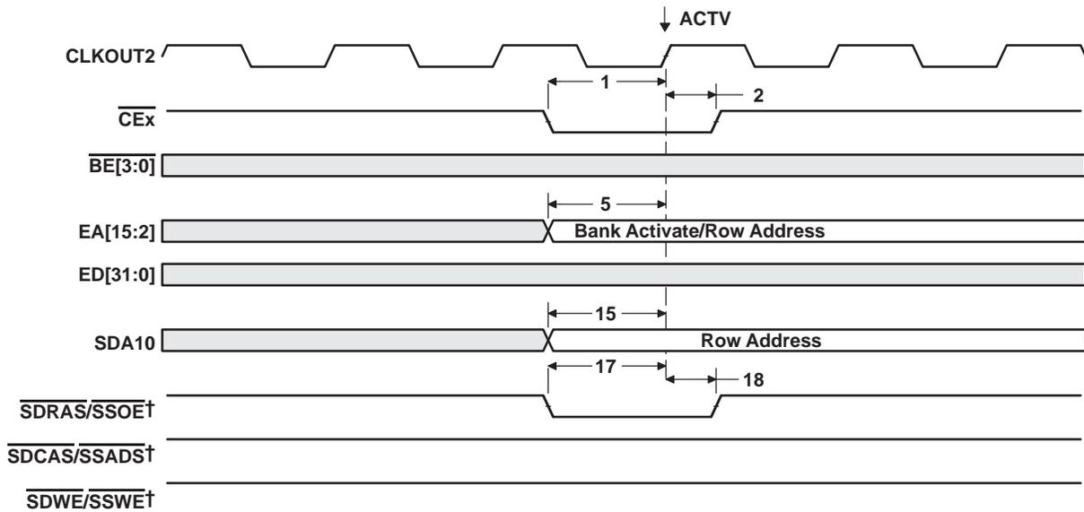
†  $\overline{\text{SDCAS}}/\text{SSADS}$ ,  $\overline{\text{SDRAS}}/\text{SSOE}$ , and  $\overline{\text{SDWE}}/\text{SSWE}$  operate as  $\overline{\text{SDCAS}}$ ,  $\overline{\text{SDRAS}}$ , and  $\overline{\text{SDWE}}$ , respectively, during SDRAM accesses.
