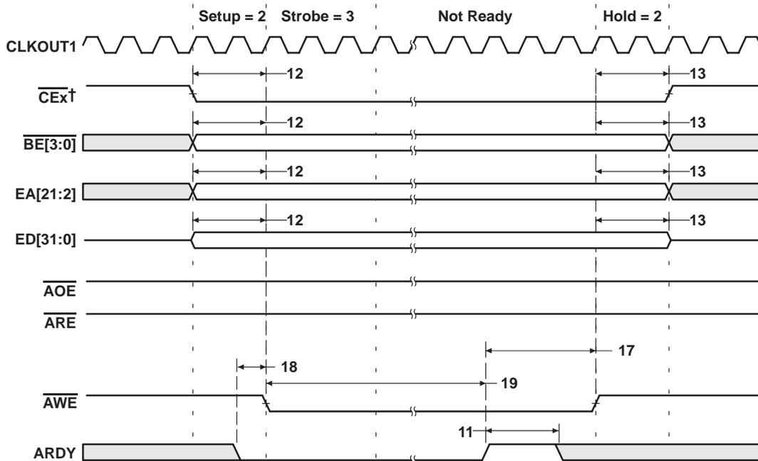
† If no write accesses are scheduled for the next cycle and write hold is set to 1 or greater, then  $\overline{\text{CE}}_{\text{x}}$  stays active for three cycles after the value of the programmed hold period. If write hold is set to 0, then  $\overline{\text{CE}}_{\text{x}}$  stays active for four more cycles. This does not affect performance, it merely reflects the EMIF's overhead.
