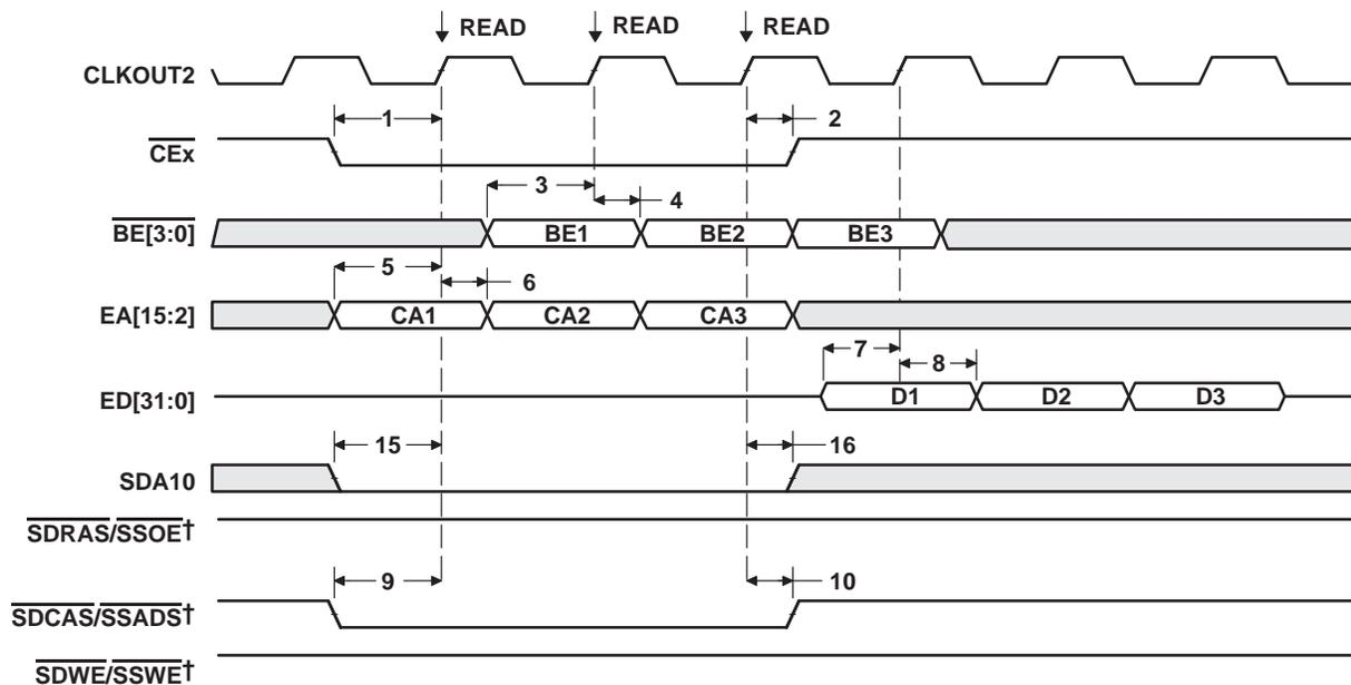
†  $\overline{\text{SDCAS}}/\overline{\text{SSADS}}$ ,  $\overline{\text{SDRAS}}/\overline{\text{SSOE}}$ , and  $\overline{\text{SDWE}}/\overline{\text{SSWE}}$  operate as  $\overline{\text{SDCAS}}$ ,  $\overline{\text{SDRAS}}$ , and  $\overline{\text{SDWE}}$ , respectively, during SDRAM accesses.
