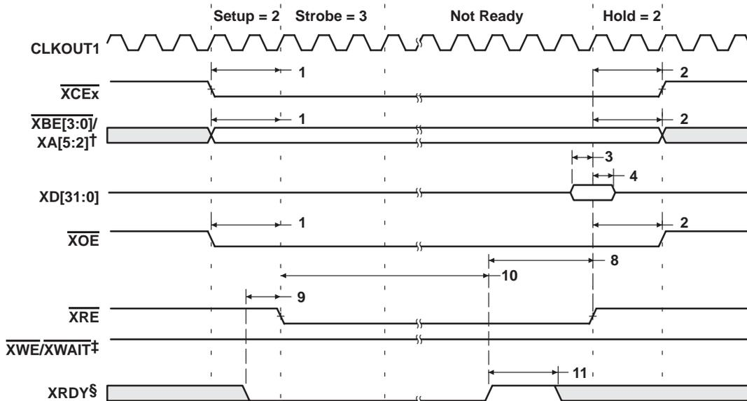
† XBE[3:0]/XA[5:2] operate as address signals XA[5:2] during expansion bus asynchronous peripheral accesses.
