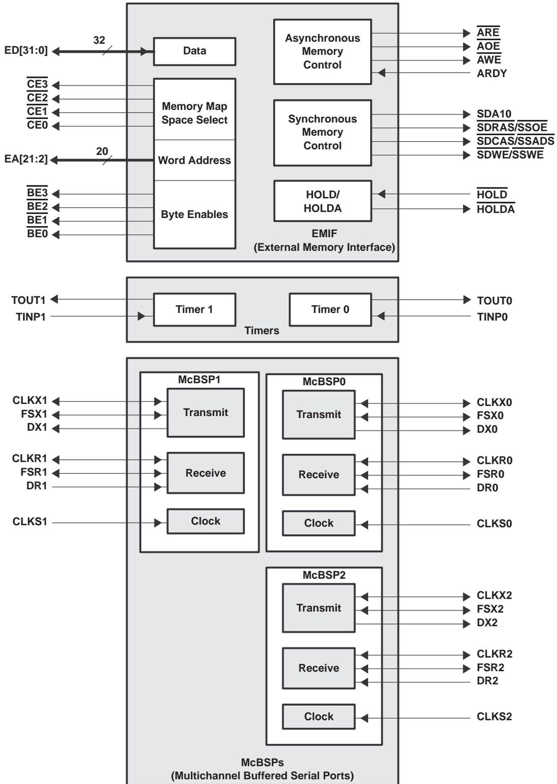
Figure 3. Peripheral Signals
