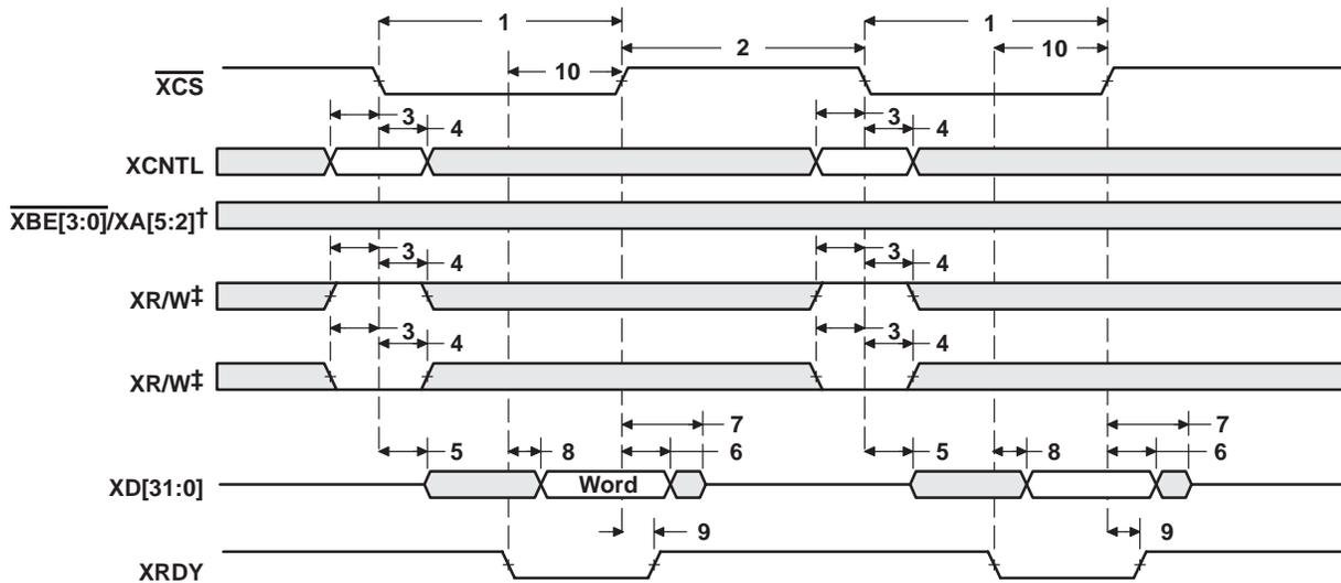
†  $\overline{\text{XBE}}[3:0]/\text{XA}[5:2]$  operate as byte-enables  $\overline{\text{XBE}}[3:0]$  during host-port accesses.
