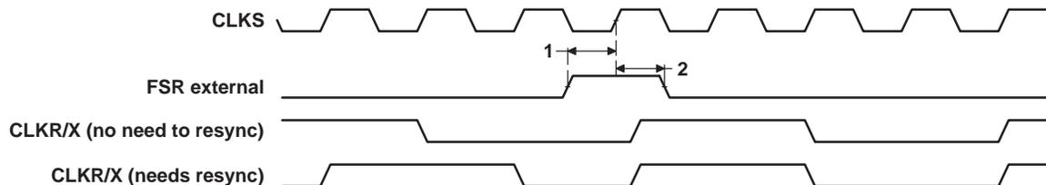
Figure 51. FSR Timing When GSYNC = 1
