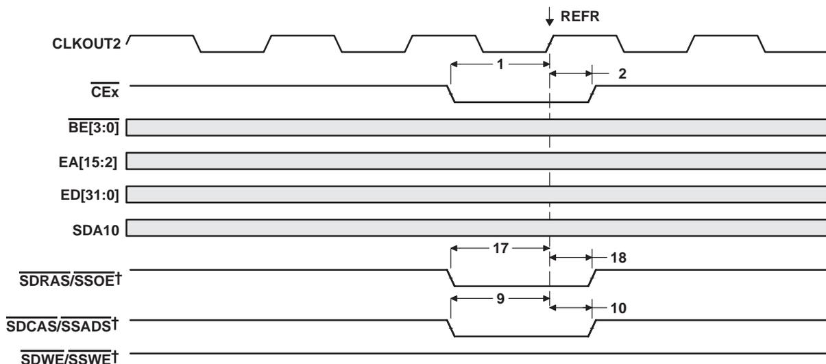
†  $\overline{\text{SDCAS}}/\overline{\text{SSADS}}$ ,  $\overline{\text{SDRAS}}/\overline{\text{SSOE}}$ , and  $\overline{\text{SDWE}}/\overline{\text{SSWE}}$  operate as  $\overline{\text{SDCAS}}$ ,  $\overline{\text{SDRAS}}$ , and  $\overline{\text{SDWE}}$ , respectively, during SDRAM accesses.
