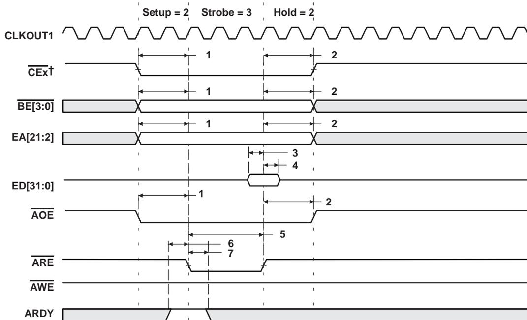
†  $\overline{\text{CE}}$  stays active for seven minus the value of Read Hold cycles after the last access (DMA transfer or CPU access). For example, if read HOLD = 1, then  $\overline{\text{CE}}$  stays active for six more cycles. This does not affect performance, it merely reflects the EMIF's overhead.
