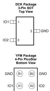
$0.8 \text{ mm} \times 0.8 \text{ mm} (0.4 \text{ mm pitch})$
