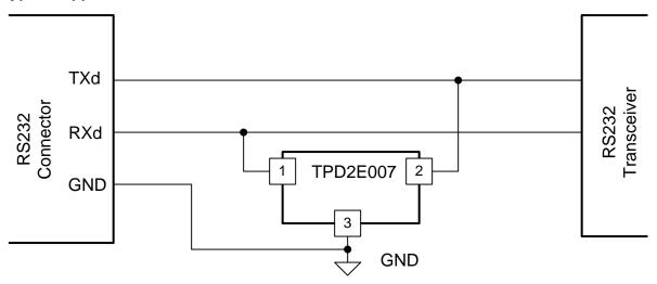
Figure 6. Example Schematic
