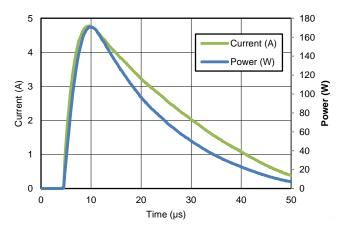
Figure 7. Surge Pulse Waveform
