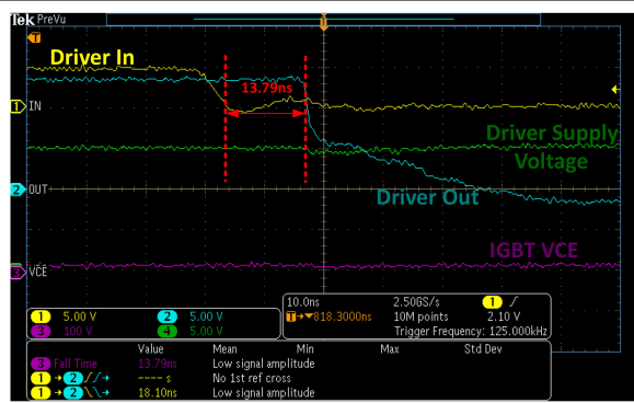
图 8-3. UCC27624-Q1 Used to Drive IGBT in the Boost Converter
